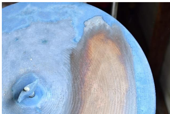
Fig. 10 On the island of La Désirade (Guadeloupe), a musician uses hydrochloric acid to clean his cymbals, which have been oxidised by gas emissions from Sargassum seaweed. La Désirade, Guadeloupe. Photo by Florence Ménez, August 2025. DOI :10.34847/NKL.68CC110Y .
